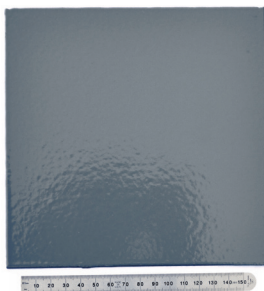
Steel plate coated with MarineLINE®, pending mechanical damage with a hammer.
