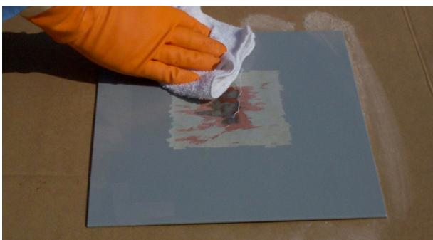
Clean the repair area with appropriate solvent. Note: Always use clean white cloth. Do not use shop rags.
