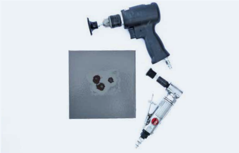
Pneumatic air drill (~ 20,000 to 25,000 RPM)
