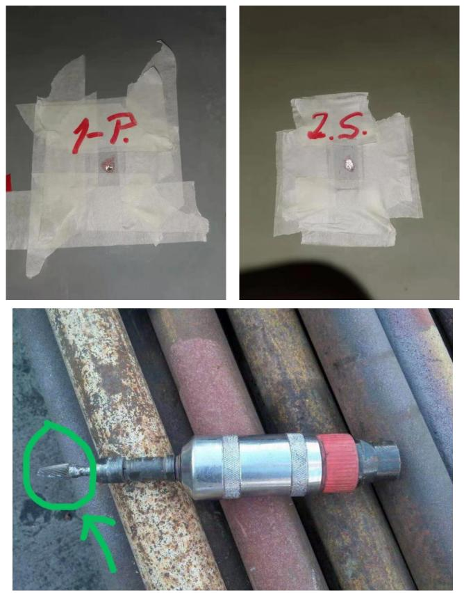
The above photo is the recommended grinding tools for the pinpoint rust area, this grinding head can make some steel profile while not enlarging the bare steel area.
